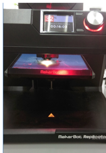
Fig. 12. The propeller at the beginning of the printing process
